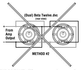
IMPORTANT: When connecting two Beta Twelve.dvc subwoofers together, use Method #1 to create a net 4-ohm impedance. NEVER USE METHOD #2, since most amplifiers cannot fully control driver movement in this configuration.
